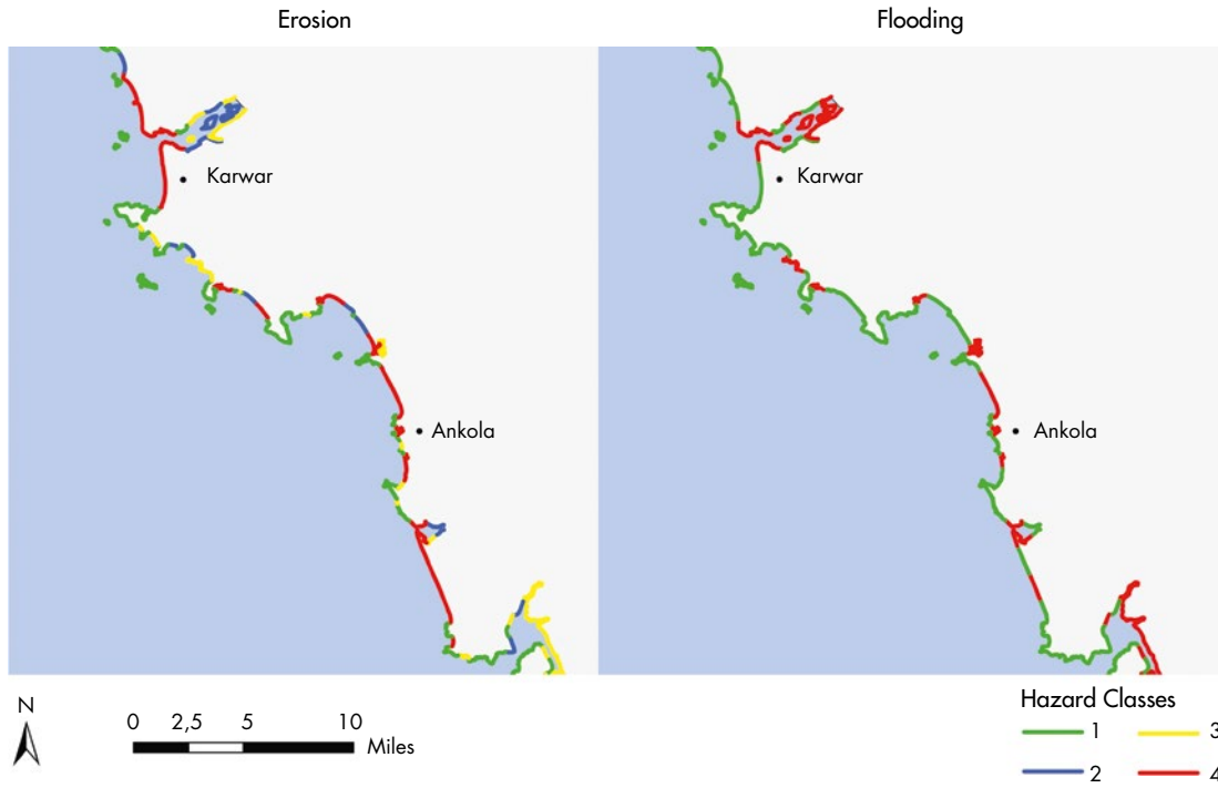
Fig. 30. Sub-regional hazard maps for northern Karnataka, India showing the hazards of erosion and flooding (Rosendahl Appelquist and Balstrøm 2015).
