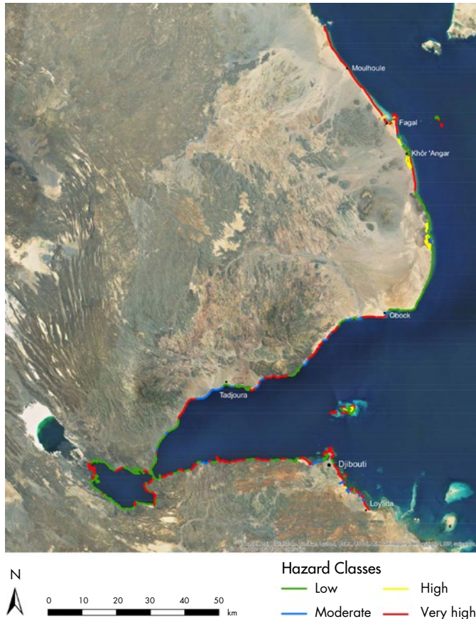
Fig. 29. National hazard map for the Republic of Djibouti showing the hazard of ecosystem disruption (Rosendahl Appelquist and Balstrøm 2014)
