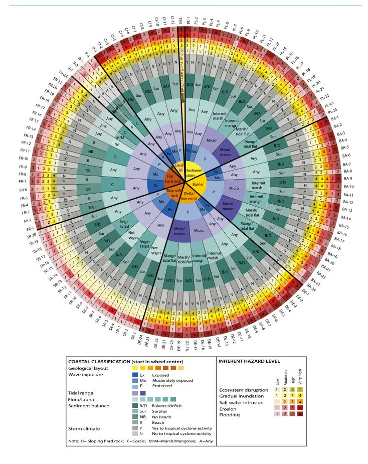
The Coastal Hazard Wheel 3.0 consisting of six coastal classification circles, five hazard circles and the coastal classification codes. It is used by starting in the wheel centre moving outwards through the coastal classification (modified from Rosendahl Appelquist and Halsnæs 2015 and Rosendahl Appelquist 2013).
